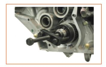
4. If necessary remove oil seal from timing housing.
