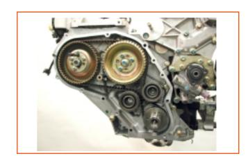
6. Install tool nr. 8130633 pin in the fuel injection pump pulley and fit it in pump flange.
