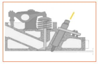
Resurfacing can be made only if the maximum nozzle projection to the cylinder head does not surpass the specified dimension (1.82 - 2.10 mm).
