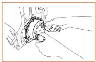
6. Flex side rods of tool nr. 8130648, pressing against crankshaft flange.
