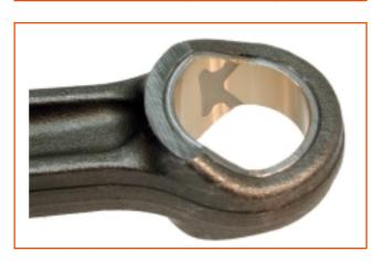
2. Assembly piston in connecting rod, with combustion chamber turned to the same side of the shell lock. Manually install pin and snap rings. If it is difficult to assembly the pin, heat the piston in water or oil at 80 °C (176 °F). The piston must be carefully handled, because any damage on its surfaces may cause bad engine operation. Assembly connecting rod and piston in the same cylinder whether they have not been replaced.
