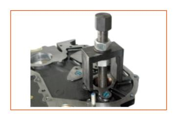
2. Remove camshaft rear seal.
