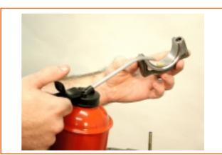
8. Assembly cap on connecting rod corresponding to the cylinder, watching blue mark on cap, bolt and connecting rod, and tighten according specified. Manually turn crankshaft when assembling each connecting rod. If it is difficult to turn, check all tightening applied in connecting rods fixation.
