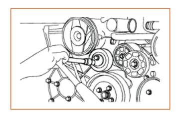
7. Remove belt from pulley handling it over the fan.
