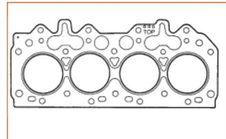
4. Select a new gasket with the correct thickness.
