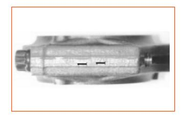
7. Connecting rod and cap have serial number on one of its side. When assembling cap, check if its serial number corresponds to the connecting rod number.
