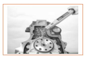
8. Carefully remove tool nr. 8130648 and check the perfect accommodation of the seal lip.
