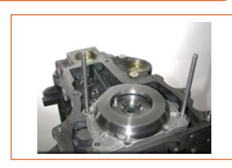
5. Install tool nr. 8130648 and turn the two rods, clockwise, fix in holes located in crankshaft flange.
