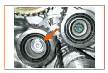
Remove distribution belt. With the use, the belt wears in the rotation sense.
