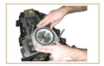
**Note:** Check seal lip positioning uniformity in crankshaft flange, avoiding edges bit.
