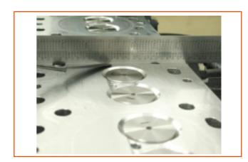
**Note:** The maximum allowed distortion is 0.05 mm; over this value, cylinder head must be
