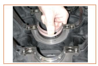
Assembly upper and lower shells on engine block and bearing caps, correctly positioning locks.
