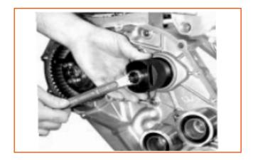
**Note:** Camshaft and injetion pump pulleys are the same, but they are assembled in inverse way.
