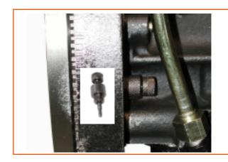
Make sure that marks are aligned (Ref. A and B) and that injection timing tool pin nr. 8130633 is correctly introduced in injection pump pulley (Ref. C).
