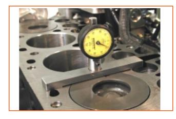
3. There are available 3 (three) types of gaskets for the cylinder head assembly, identified by holes in the left side, from front viewing.
