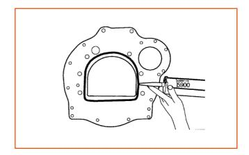
Install housing on engine block and fix it with bolts according removed and tighten according to specification, see TECHNICAL SPECIFICATIONS.
