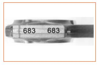
On one of the sides, connecting rod has the code of weight, that goes from, approximately, 1259 to 1322 grams and it is identified only by the two last weight digits, by an ink mark on the body of the connecting rod.
