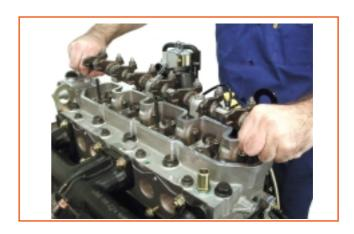
3. Remove camshaft push rods marking them to reinstall in the same position later.
