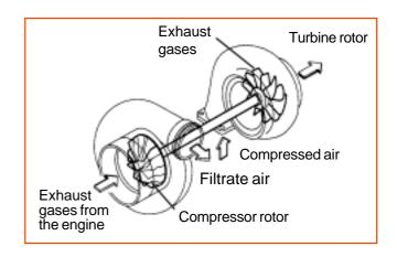
The intake of strange objects, even smalls, will damage the rotor of the compressor, damaging the operation of the turbocharger, this way, between the recommended periods check the air filtering system.
